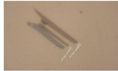
Optical image of WSe 2 : before scanning probe lithography
