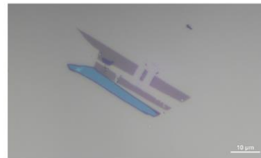
Optical image of WSe 2 : after scanning probe lithography
